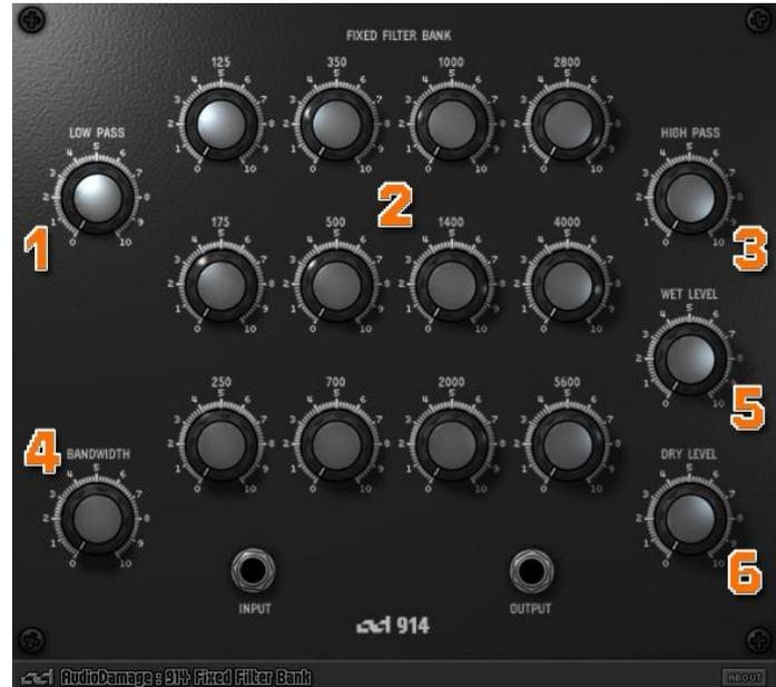
pass filters. Each knob is labeled with the center frequency of its filter. The frequencies are 125, 175, 250, 350, 500, 700, 1000, 1400, 2000, 2800, 4000, and 5600Hz. Each knob controls the loudness of signal content with frequencies near these center frequencies.
