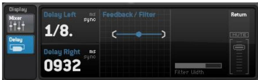
The **DELAY LEFT** and **DELAY RIGHT** controls change the amount that signals are delayed in relation to the original (dry) signal. Each delay has a range of 0 to 1999 msec, or approximately two seconds.
